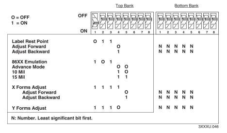
**Configuration DIP switch settings:** This illustration shows the Test and Service mode DIP switch settings for changing the configuration commands.
